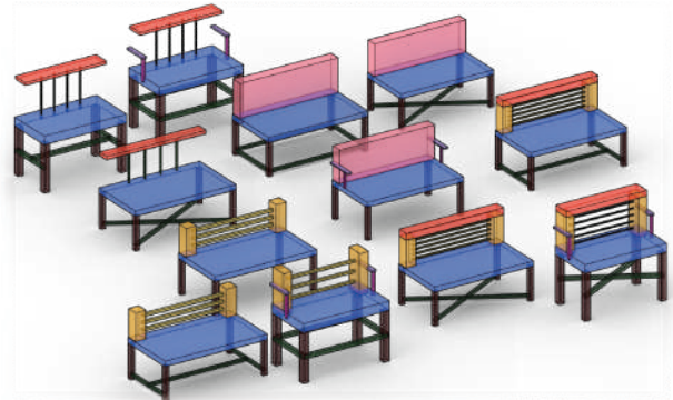
Figure 9. Synthetic chair variations. We show a few examples of the 96 structural variations of a bench, including variations to the legs, base, backrest, and armrests.
